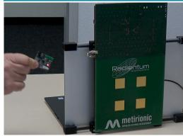
**Reflector:** Tag with PCB antenna. The size of PCB board is 4.1cm x 3.5cm. The position information of reflector relative to initiator is provided by computer connected to initiator through USB. The raw sampling data can also be provided with different configurations in the positioning system (raw data, angle + distance, position,..).
