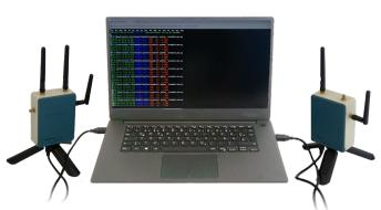
The DMK-215 Demo Kit is a plug-and-play kit that allows to gain experience with Metirionic's ranging technology.
